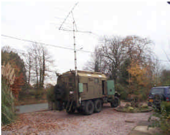
Picture right : The truck roof showing left to right the aerial storage lockers, The new VHF 2m collinear on top of the log-periodic (in green bags) and the flexible exhaust extension for the generator.
